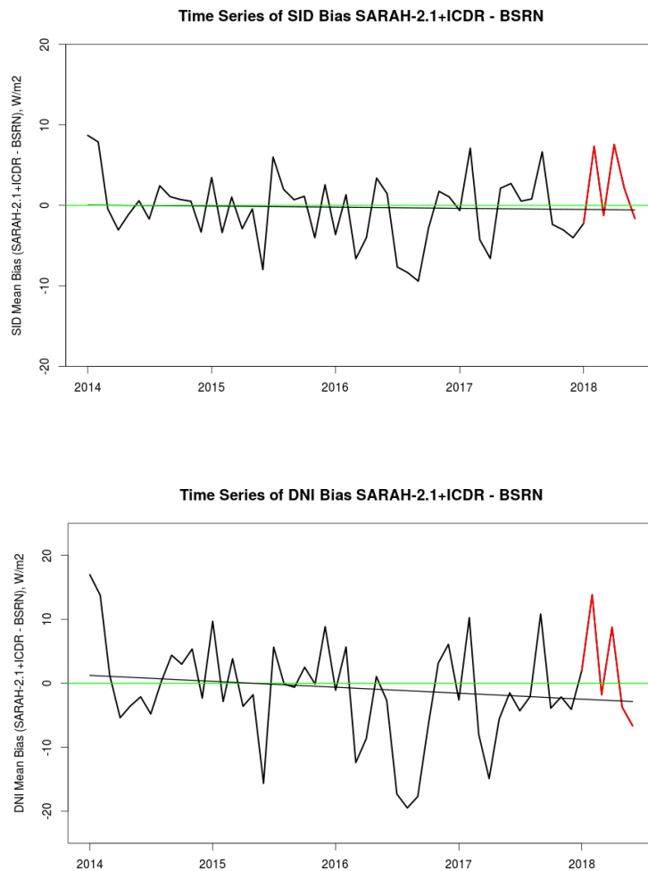
Figure 3-4: Bias time series of the SDI parameters SID (top) and DNI (bottom) of the combined CDR SARA-2.1 and ICDR SEVIRI Radiation data with reference to BSRN reference stations for the time period 2014 to June 2018.
