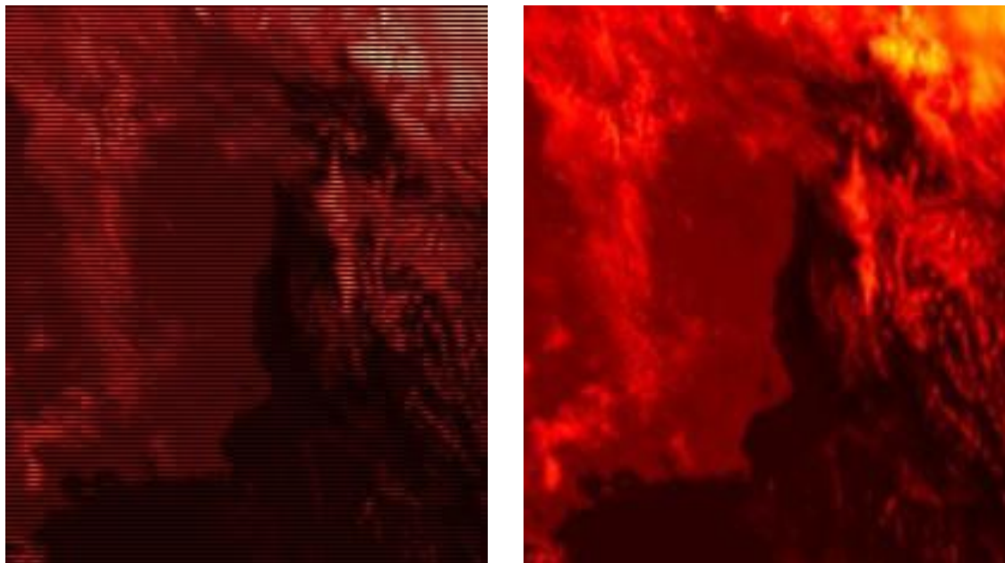
Figure 27: Example of the effect of stripes interpolation. Earth disk's area for day 1985.12.01 at 12:00 (MFG-2) before (left) and after (right) interpolation.
