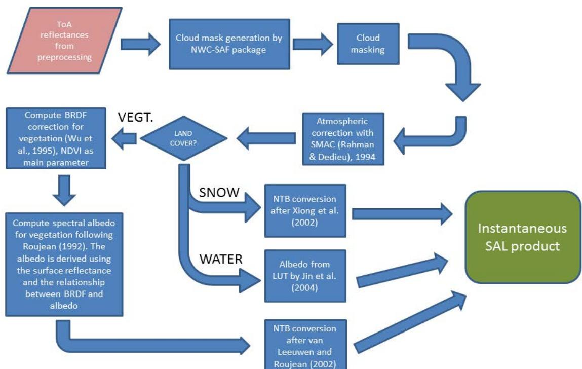
**Figure 2: The process flow of the CLAAS-SAL product computation.**
