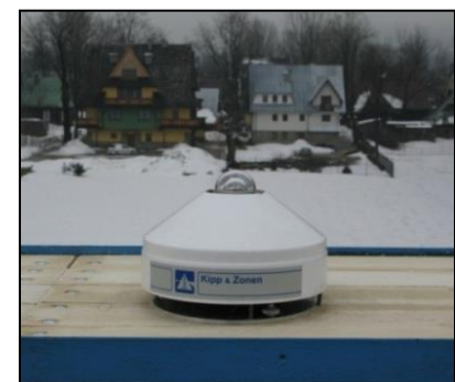
Kipp&Zonen CM6B Pyranometer supplied with ventilation fan and heater [Zakopane]
