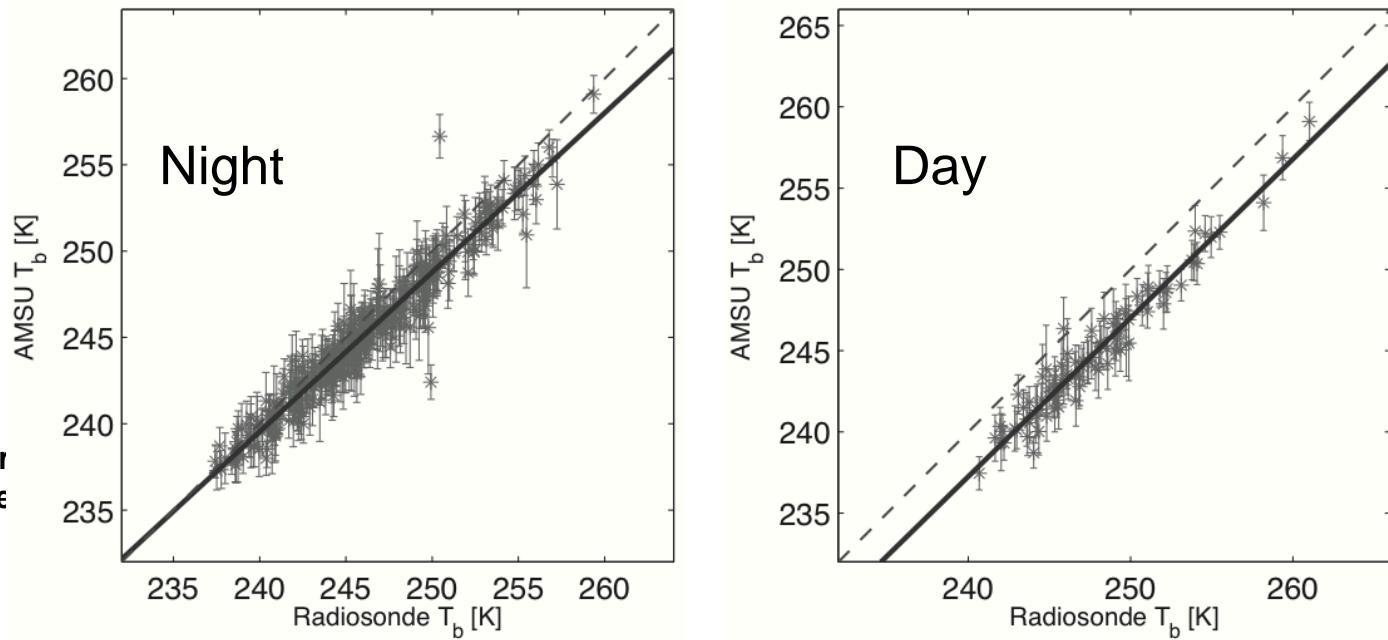
Radiosonde radiation bias, ARM Station TWP-C1
