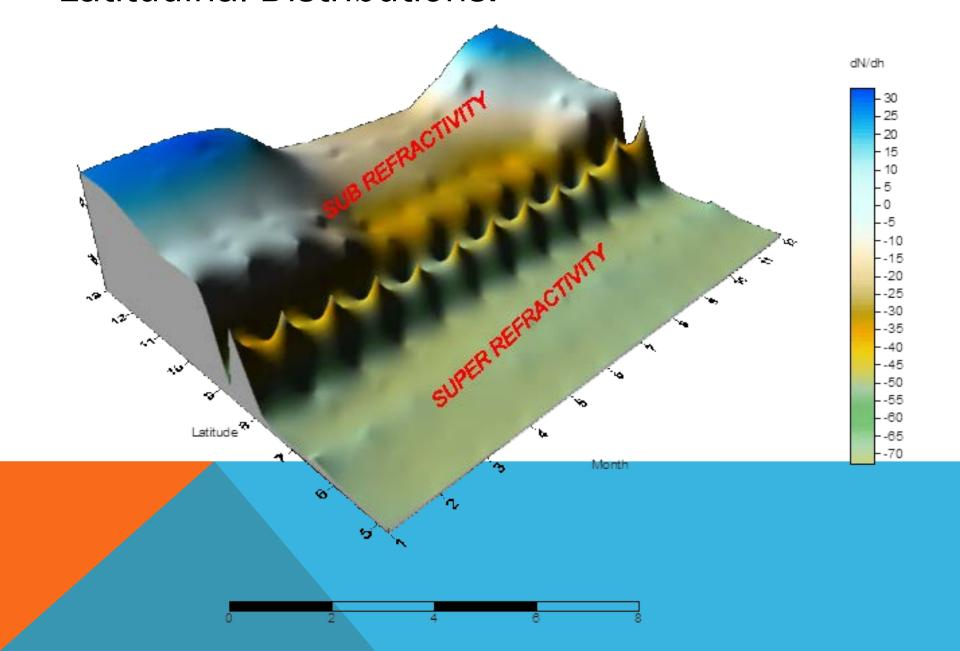
Figure above shows that between latitude 4° and 8° N, consisting of the coastal and guinea savannah regions, the atmosphere is super refractive while between latitudes 8° and 13° N, consisting of both the midland and sub-sahelian regions, the atmosphere is sub-refractive.
