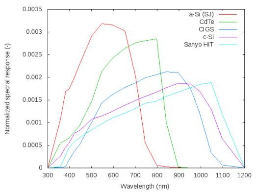
Normalized spectral response curves for 5 different modules, measured at the ESTI laboratory
